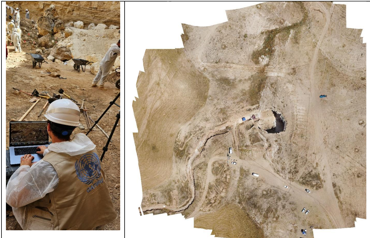
Figure 007- Unmanned Aerial Vehicle (UAV) Capture of Sinkhole at Bir Alou Antar and it's environs. Post-Processed mosaic on the right.
