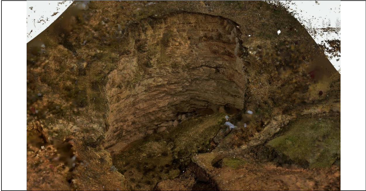
Figure 009- High-Resolution Terrestrial Laser Scan of Bir Alou Antar Sinkhole.
